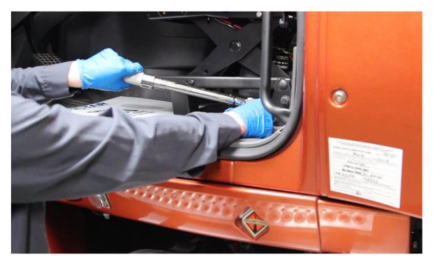
Attach the 3-point belt anchor to the ICP bar using a new bolt and flange nut, and torque them to the proper specification.
