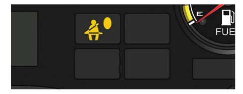
Vehicles equipped with the RollTek Rollover Protection System will include a dedicated diagnostic lamp on the dash panel.
