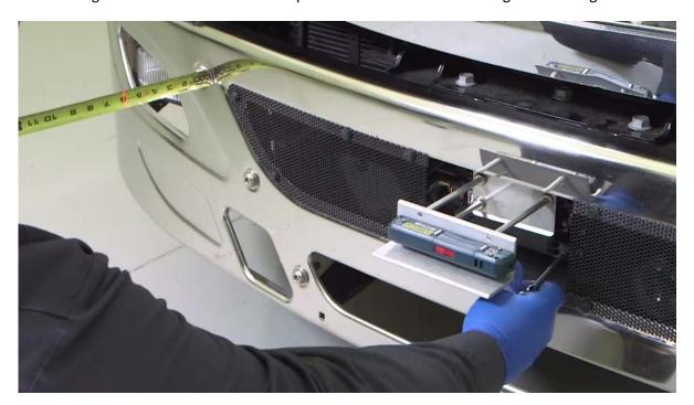
Locate symmetrical points on the front of the vehicle that are at least 12 inches (30 mm) from the vehicle's center line. Using a ruler or tape measure; measure the distance between the laser light line and the vehicle. Repeat this measurement on the opposite side of the vehicle. Compare the left and right distance measurements. A properly aligned radar sensor will have the same measurement on each side.
